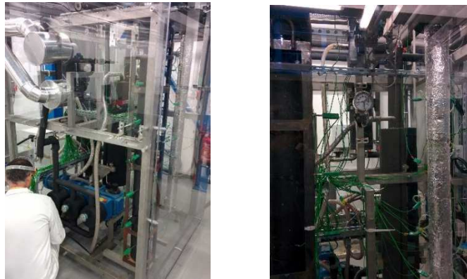
Fig. 7. Photographs of CO 2 loop and two vertical test sections
